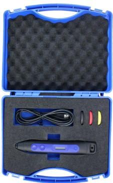
This inovative MultiPEN can read LF, HF and UHF tags and transfer data via Bluetooth or USB connection to a host computer (tablet, laptop or smartphone). Thanks to its memory, the MultiPEN can even transfer information later to the host computer.
