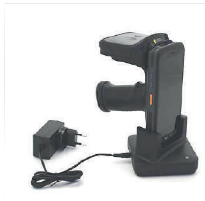
Charging cradle compatible with protection case, with charger, EU/US plug
