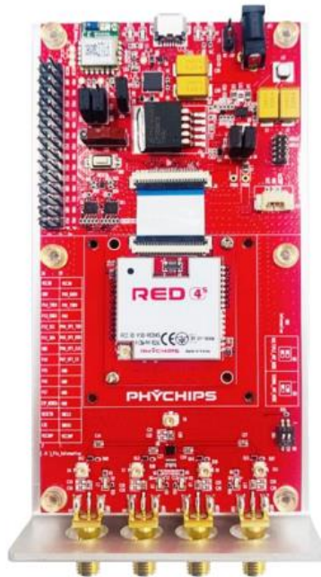
Figure 1. RED_CTRL with RED4S module
