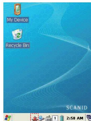
After Bluetooth executed, the Bluetooth BTPAN1 icon will be appeared on the bottom of Windows Taskbar, and the red cross mark on it shows that you access is available and prepared to be accessed.
