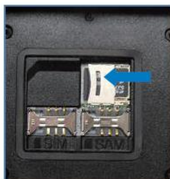
Push the cover up as arrow direction to lock it, and attach the main battery and turn on the power.
