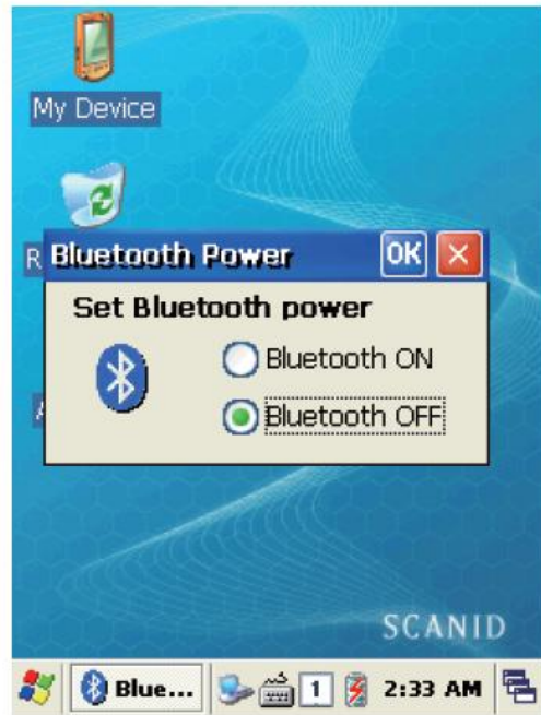
Select "Bluetooth OFF", then to press OK button to off the Bluetooth power.
