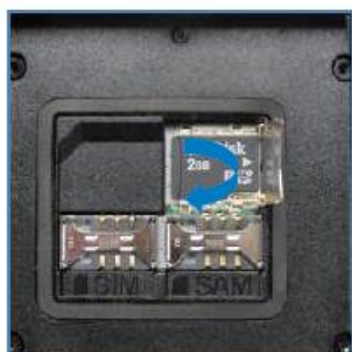
Put Micro SD card into Slot and press down the cover as arrow direction.
