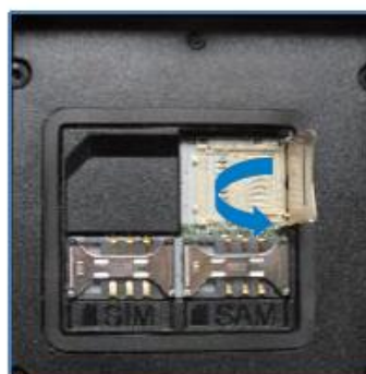
lift the cover up along arrow direction.
