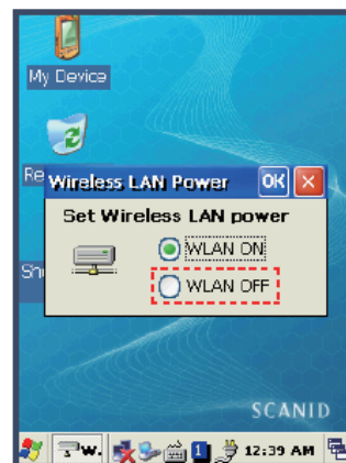
Start Button/Programs/ ATID App/Wireless Lan, and then select <OFF> to stop Wlan communication.
