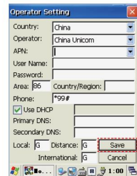
If there is the SIM card, then setting each item on the Operator Setting interface, and press <Save> button
