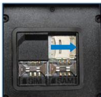
Push the cover to the right along arrow direction to open it.
