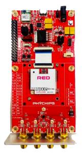
The Developer Kit by Phychips is easy to test and use with RED 4s. This OEM RFID UHF module offers superior performance, small form factor and advantages in time-tomarket to customers.
