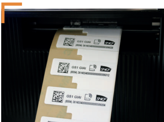
GIAI encoding and impression of an AX'Label Platina RFID label with TOSHIBA printer
