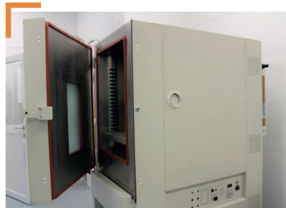
Climate chamber to test the environmental resistance of tags
