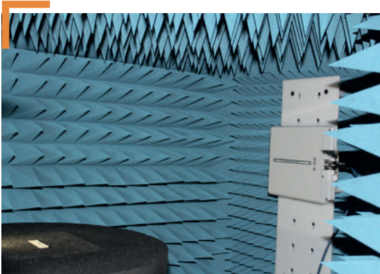
Anechoic chamber to test tag reading performance
